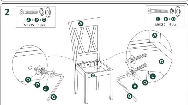
Attach "P"and "O" washers to "J" bolt. Connect the seat frame "D" to back fame "A". Use the bolts to attach.
