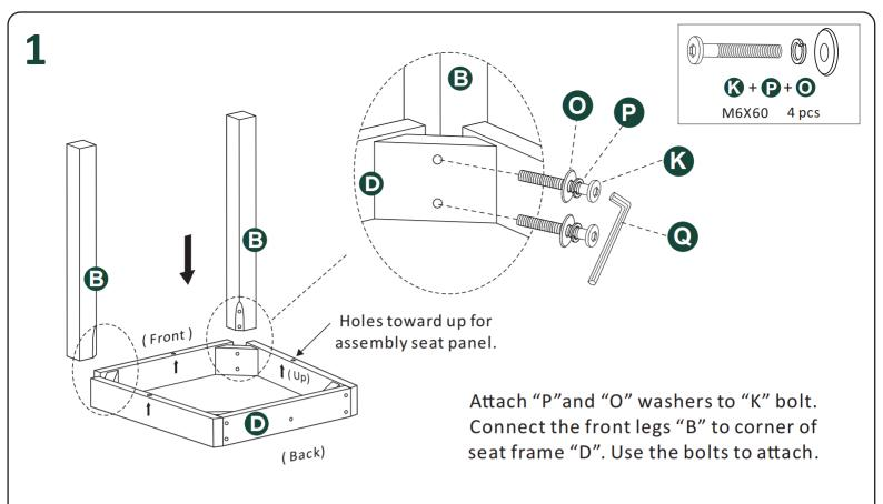
IMPORTANT: To best ensure a steady chair with no wobbling, partially tighten all bolts first, ensure alignment of parts being connected, then fully tighten bolts. Should the chair wobble upon assembly (rare) loosen bolts as needed to adjust alignment and then retighten bolts.
