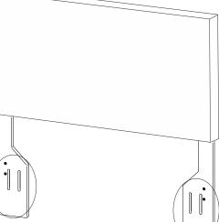
To attach hook-on side rails to the headboard, first insert 2 pcs M8 x 20 bolts (not included) into the holes on the outside of the slots of both headboard legs. Then slide the hooks on the ends of the rails over the bolts in the headboard legs.
